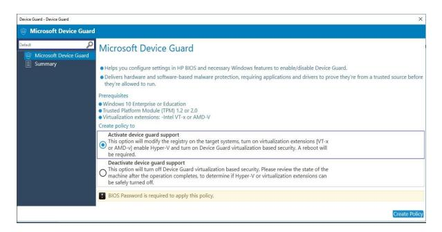
**a.** Create a policy to activate device guard support—Modifies the registry on target systems, enables the virtualization extension, enables Hyper-V, and enables Device Guard virtualization-based security.
